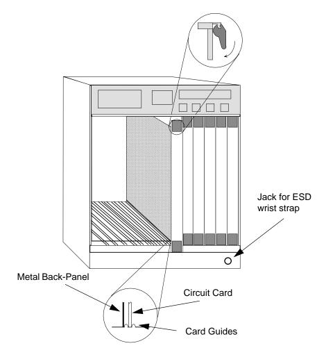
Warning: Ensure that the circuit card is between the card guides. Lock down the top and bottom plastic tabs at the same time, applying even pressure.
